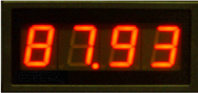
1/8 DIN standard size, 4 DIGIT 0.8" LED
